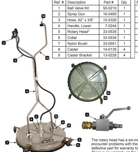
AW-7020-8007 Ref. # Description Part # Qty. 10 Cover 33-0552 1 11 Mounting Blocks 56-0072 2 43-0140 1 12 Pin and Ring Set 13 7-0243 1 Handle, Upper 14 Hand Grip 7-0237 1 15 Rotary Arm 33-0553 1 3 16 Nozzle, 25 Deg. 020 18-0298 Head Rebuild Kit 70-0598
